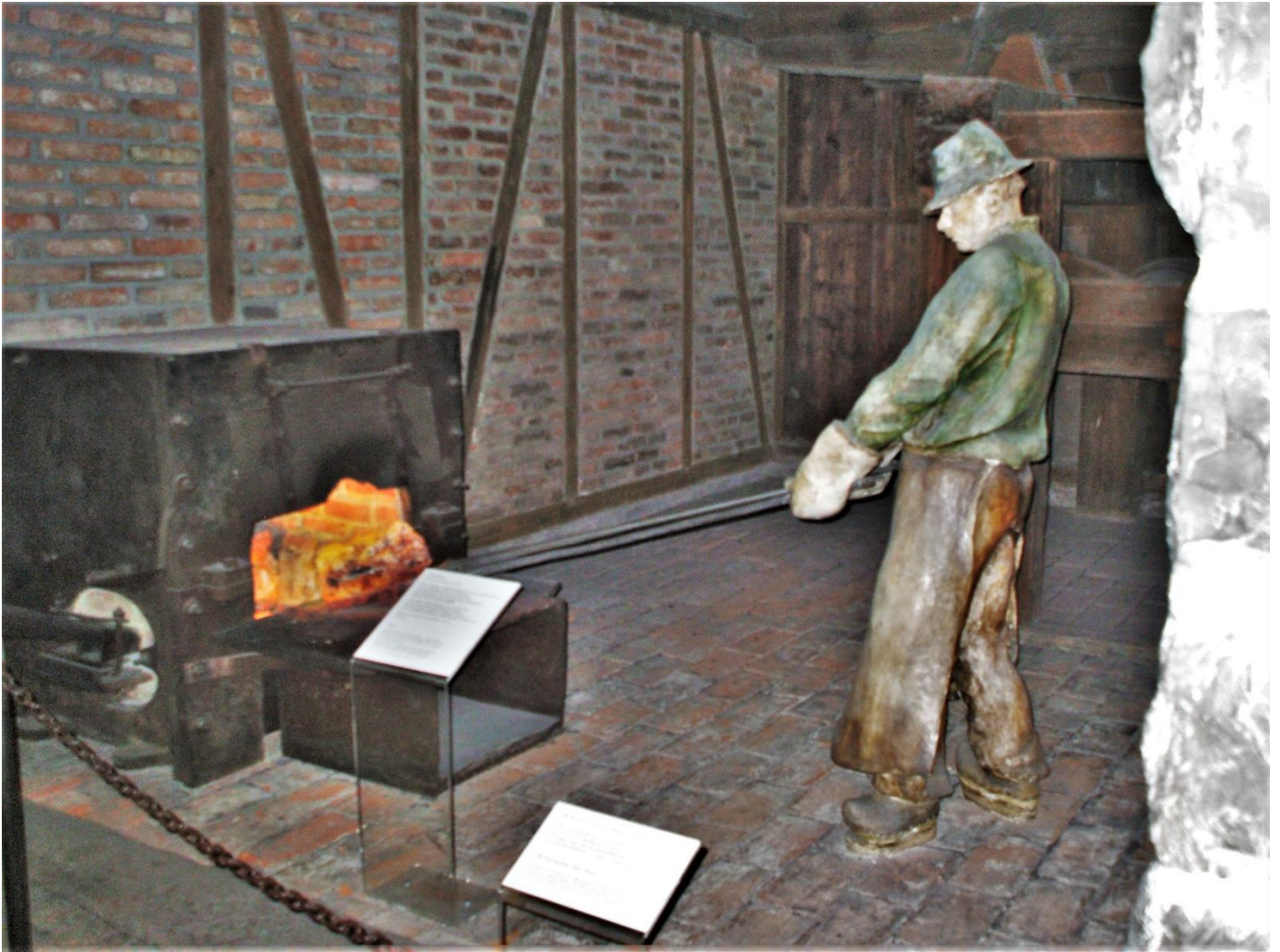
Fig 8 : Display 3 showing the removal of the ball from the puddling furnace
