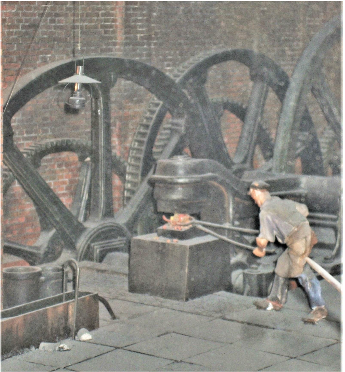
Fig 5 : Display 1 , showing the shingling hammer
