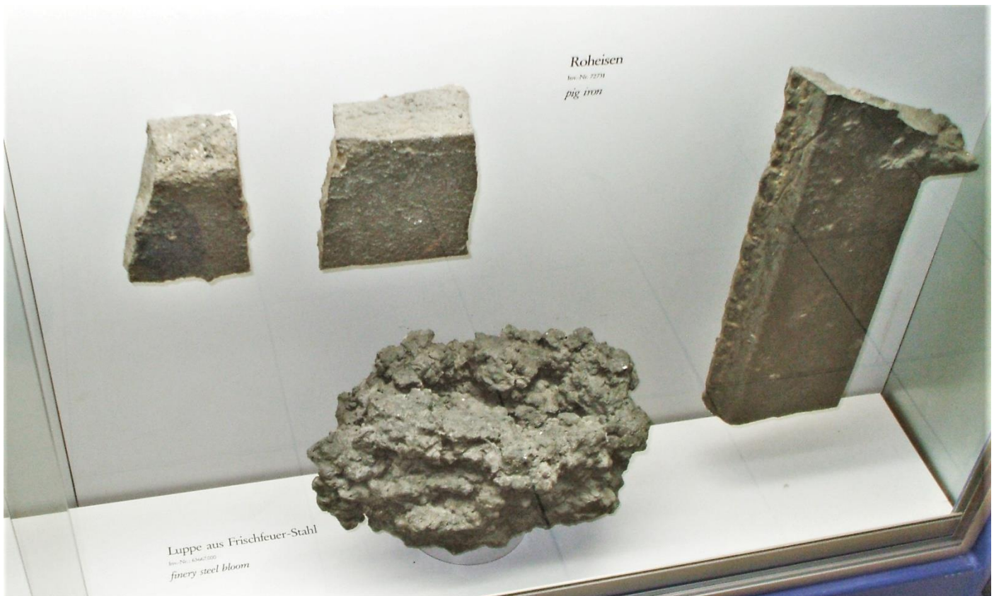
Fig 13 : Display 4 showing examples of fractured pig iron and “steel” made by puddling
