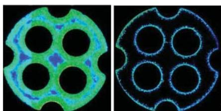
Fig. 9. Relative concentration of nickel on cross sections of QUADRALOBE<sup>TM</sup> shaped pellets, comparing KATALCO<sub>JM</sub><sup>TM</sup> 57-4Q against KATALCO<sub>JM</sub><sup>TM</sup> 57-6Q. The brighter spots represent a higher concentration of nickel
