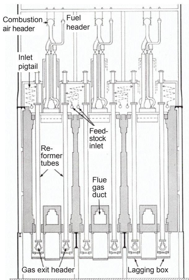
Fig. 2. Drawing of the first steam reformer in Billingham 1936 (Reproduced with permission from (2))
