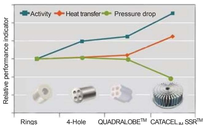
Fig. 8. Plot of CATACEL<sub>JM</sub> SSR<sup>TM</sup> relative performance of different catalyst types (14)
