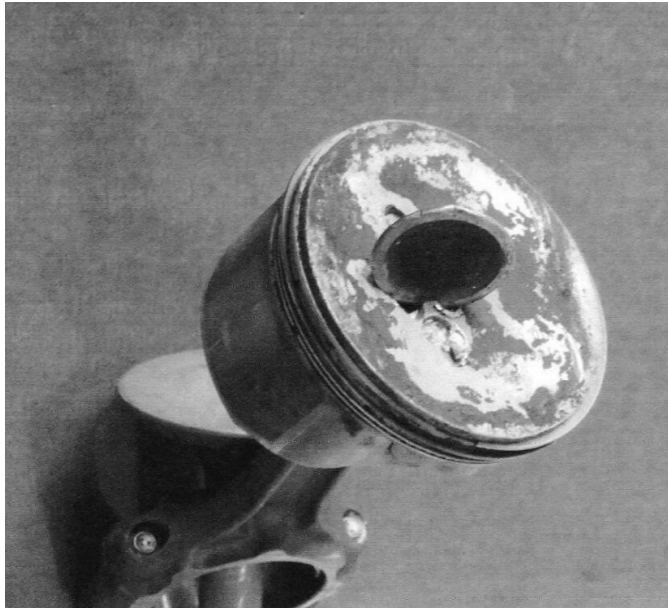
Figure 7. Valve Crown has embedded itself in the Piston
