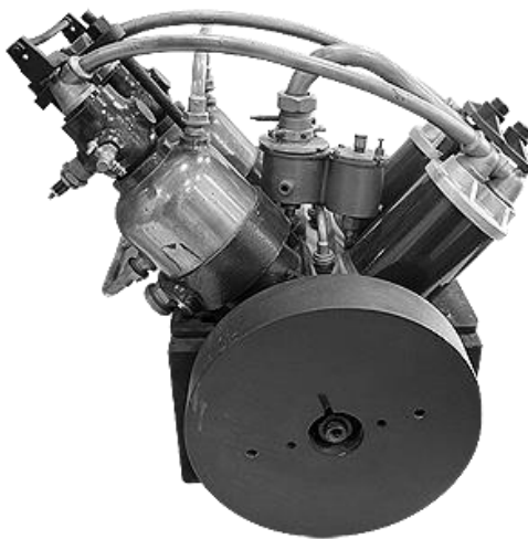
Figure 3. The two-stroke Dolphin engine.
