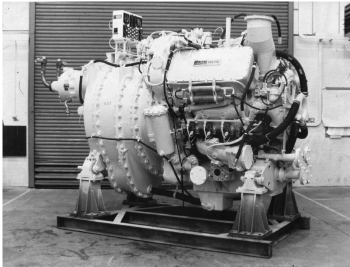
Figure 15. An E280 all non-magnetic parts, nine-cylinder propulsion Deltic, the D9-59K giving 950 bhp at 1700 rpm to Royal Navy Mine Counter Measure Vessels of the “ Hunt Class ”.
