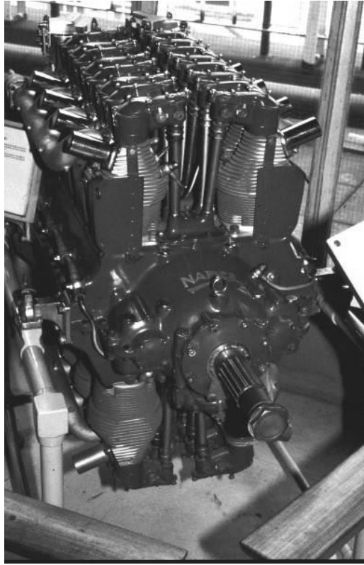
Figure 7. Of “H” layout with two crankshafts and 16 air cooled cylinders, the lighter “E93” NAPIER “Rapier” 380 bhp aero engine of 1932 had 32 push-rod operated overhead valves.
