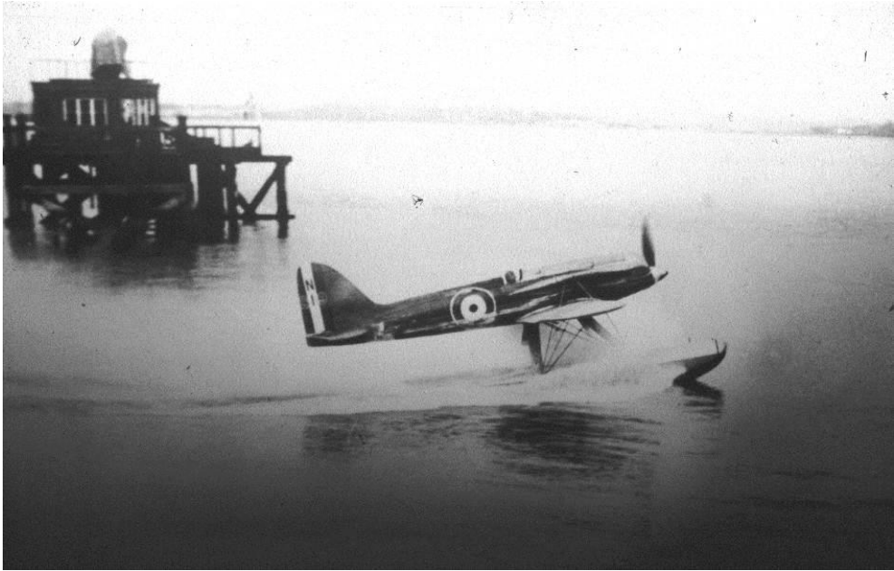
Figure 5. The Schneider Trophy winning Supermarine "S5" in 1927, powered by a reduced frontal area "Racing Lion 7B" of 875 bhp.
