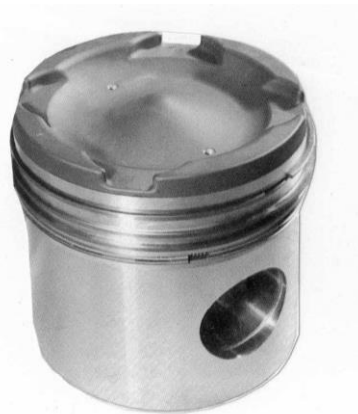
Figure 11. An early RK270 piston with a four piece ring set and hard anodised crown to improve thermal fatigue resistance
